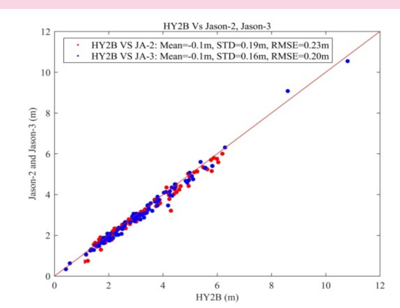
Results relatively to the 2 altimeters are very good. Standard deviation of differences is about 20 cm. The root mean square error (rmse) ranges from 20 cm to 23 cm. The bias is negative.
