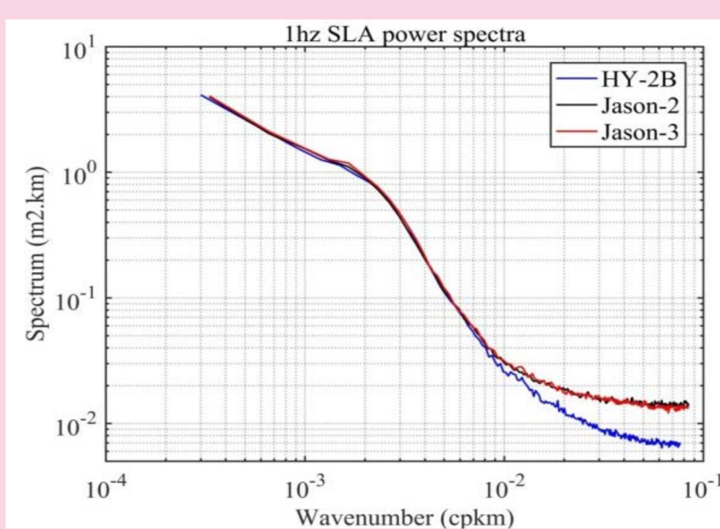
We note that the noise floor for the 1-Hz data from HY-2B is smaller than JA2 and JA3.
